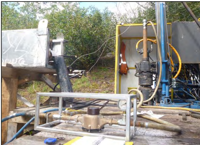
PHOTO 66 MW16-003 Nitrogen Packer Flowmeter Assembly
