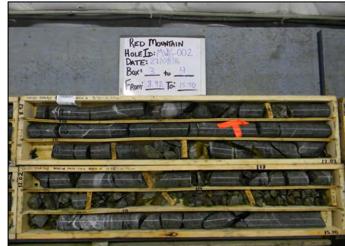
PHOTO 85 MW16-002 - Box 3-4 - 8.92-15.70 m
