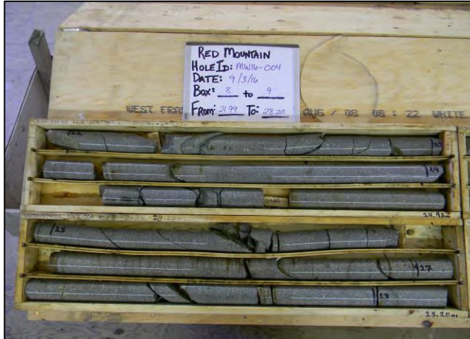
PHOTO 98 MW16-004 - Box 8-9 - 21.99-28.20 m
