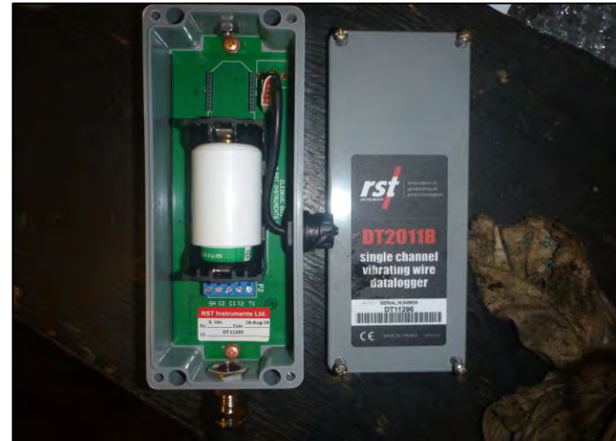
PHOTO 36 BH16-007 VWP Datalogger
