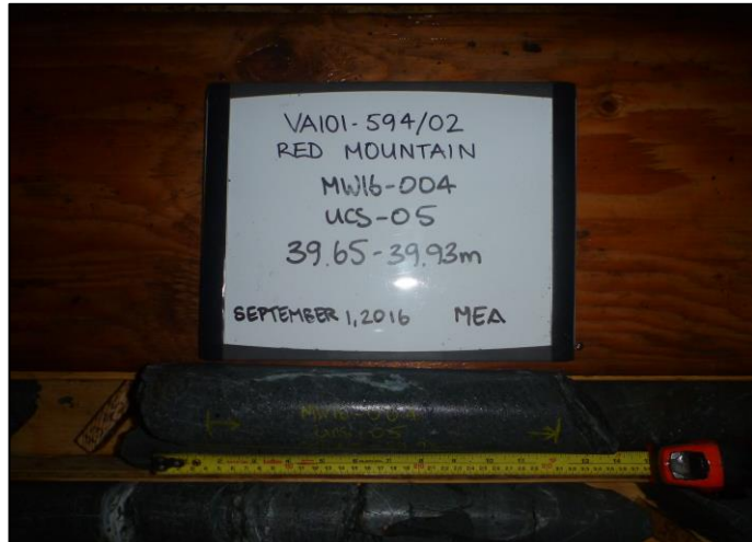
PHOTO 57 MW16-004 UCS-05 39.65-39.93m
