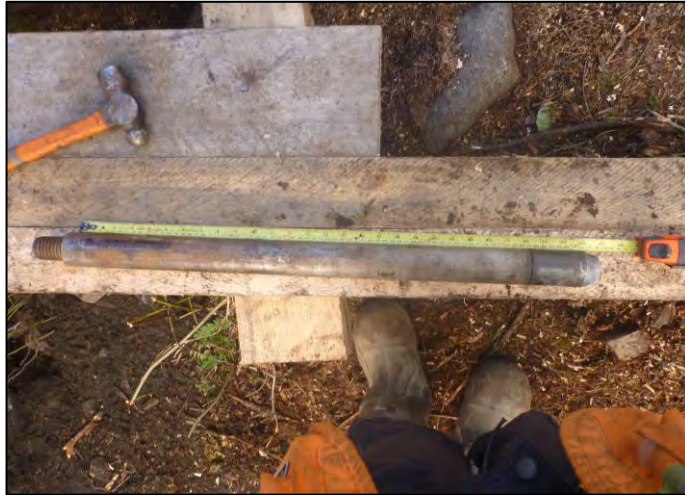
PHOTO 21 BH16-004 SPT Split Spoon Sampler
