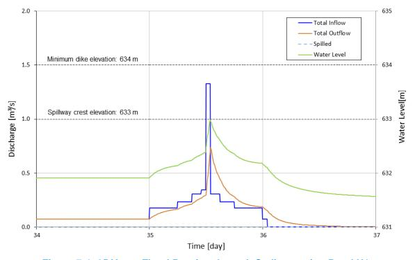
Figure 7-4: 25 Years Flood Routing through Sedimentation Pond H1
