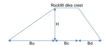
Figure 7-2: Rockfill Dike Cross-Section Sketch
