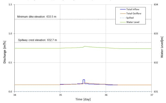
Figure 7-6: 25 Years Flood Routing through Sedimentation Pond H3
