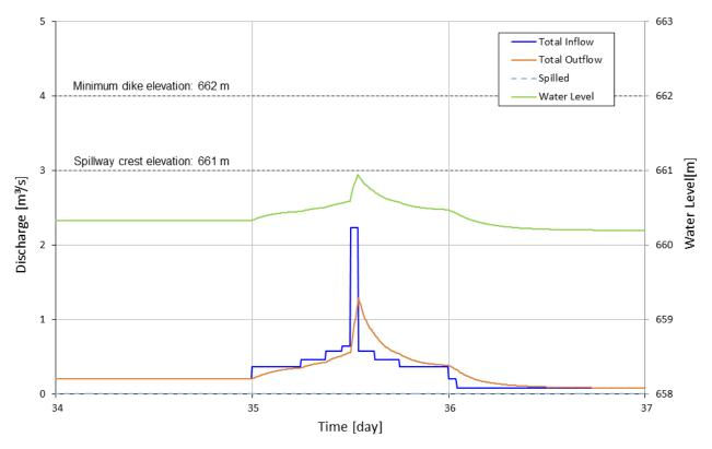
Figure 7-3: 25 Years Flood Routing through Timmins 4 Sedimentation Pond 3
