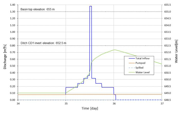
Figure 7-1: 25 Years Flood Routing through the Transfer Basin
