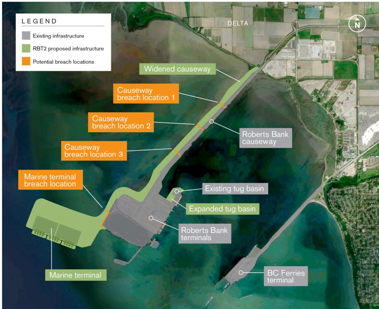
Figure IR2020-2.2-1: Potential breach locations evaluated for reducing potential disruption of juvenile salmon migration
