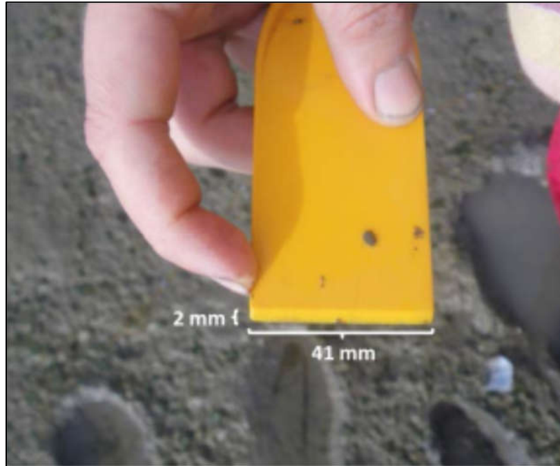
Figure 2-4 Plastic Putty Knife (with dimensions) Used for Scrape Samples
