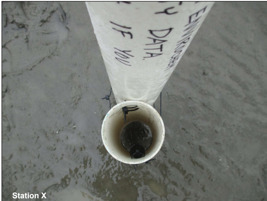
Figure 2-7 View of Sensor within Housing at the Sediment-Water Interface
