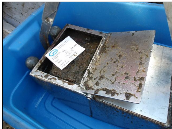
Photo A1-2: Ponar containing sediment sample. (09-14-2025)
