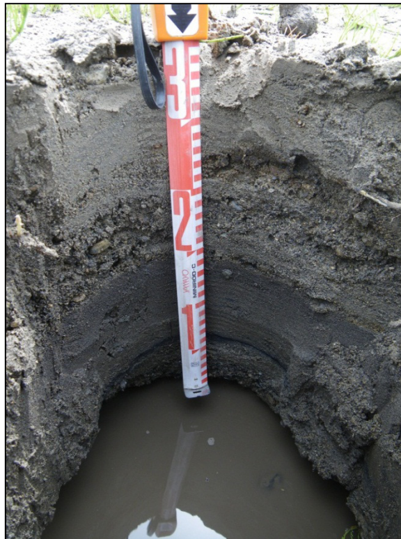
Plate 4.3-10. The imperfectly drained Gleyed Regosols often contain a high proportion of coarse fragments.
