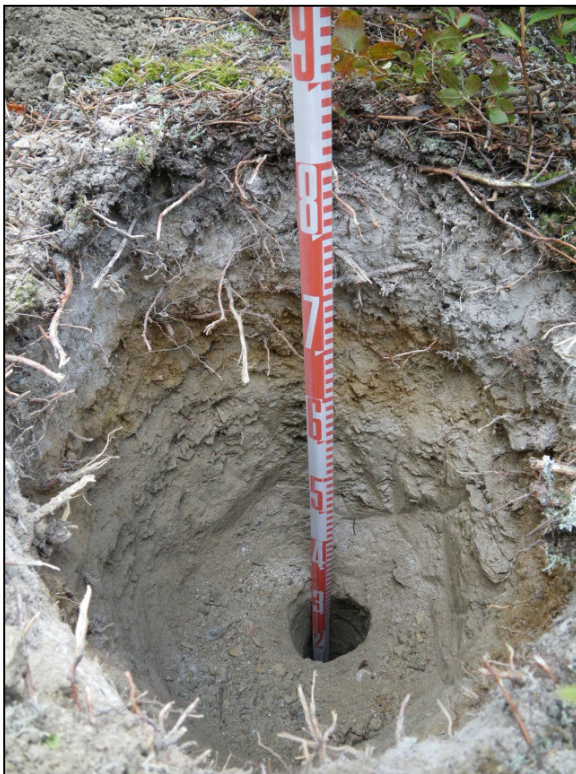
Plate 4.3-19. Typical SMU-M1 soils include well- to moderately well-drained Eluviated Eutric Brunisols with high proportion of coarse fragments.
