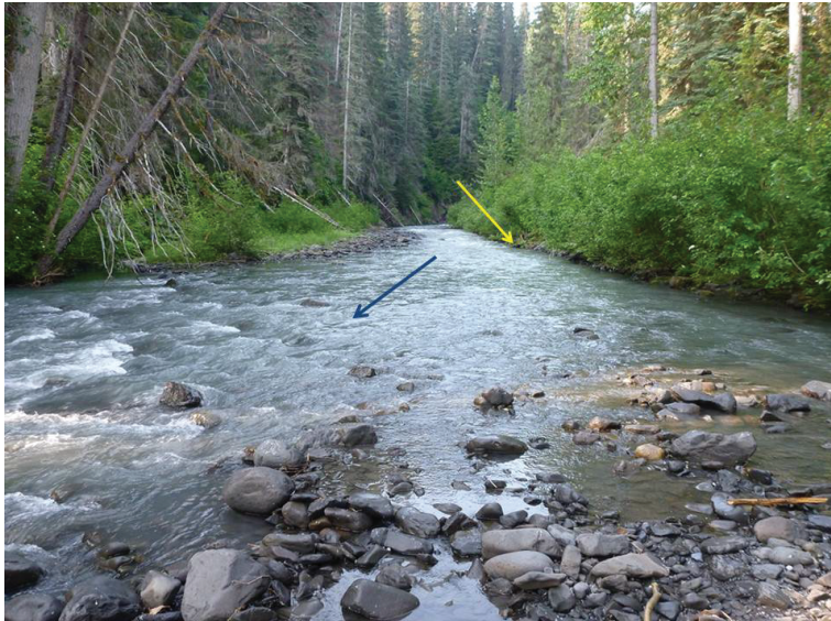
Wildfire-Hydro, looking upstream at monitored reach. Channel is bordered by low, cobbled banks and is approximately 15 meters wide during high flow events. Flow direction given by blue arrow, pressure transducer located at yellow arrow. Photograph taken on July 26, 2012.
