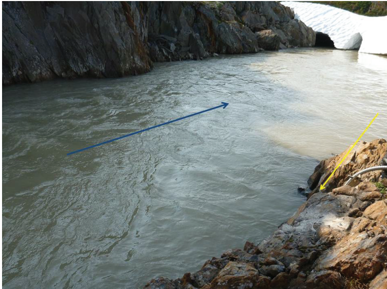
BNL-H1a pressure transducer location. The channel is approximately 9 meters wide and is constrained by steep bedrock walls for this low gradient reach. Blue arrow gives flow direction and yellow arrow indicates pressure transducer installation. Photograph taken on July 24, 2012.
