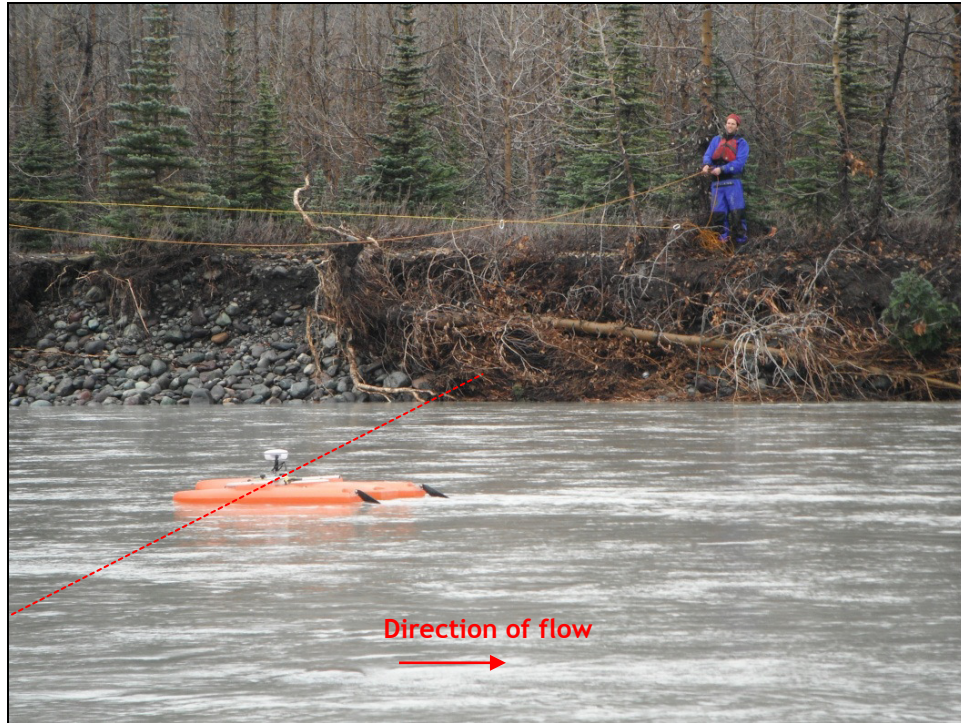
Plate 6.4-1. An ADCP measuring discharge on the Bowser River under swift water conditions. A cableway pulley system was used to guide the unit across the channel. October 26, 2011.
