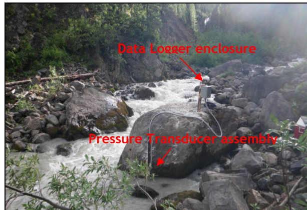
Plate 6.2-1. Low angle oblique view looking across Scott Creek towards the location of the installed hydrometric station (Scott-Hydro). July 3, 2010.
