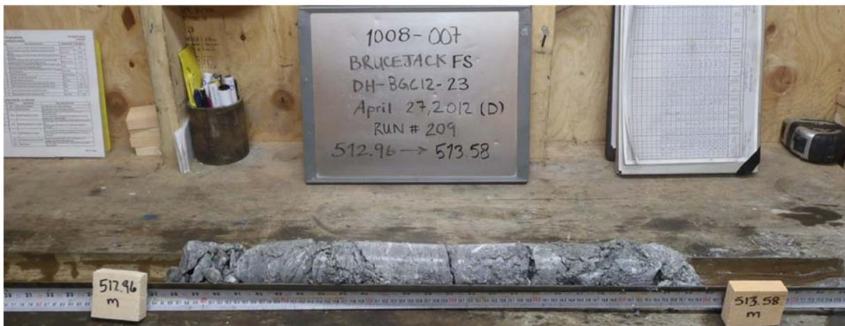
**Photograph G-4. Example of 'Worst Case' Fault-Disturbed Rock in DH-BGC12-23 (SU-318).**
