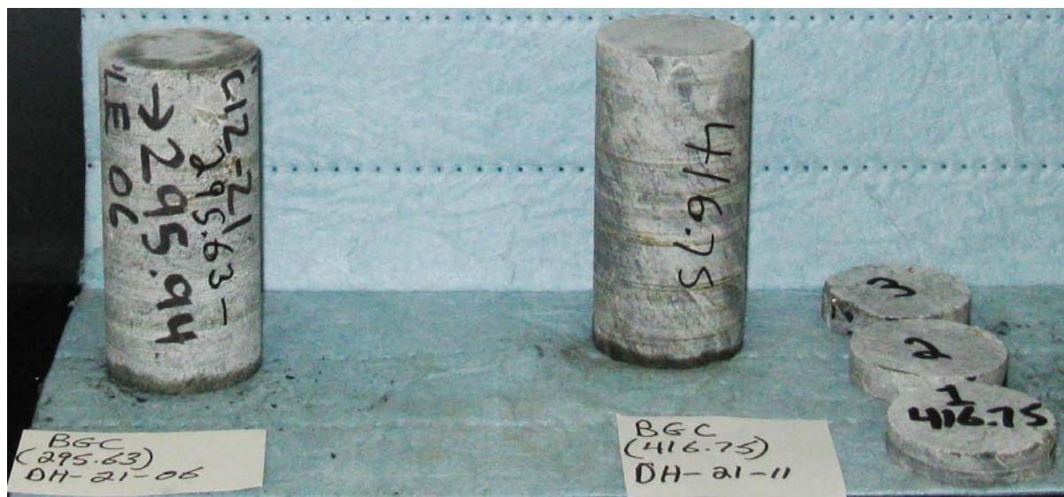
Post-Test UCS, Triaxial Confined and Brazilian Tensile Test Sample Photographs
