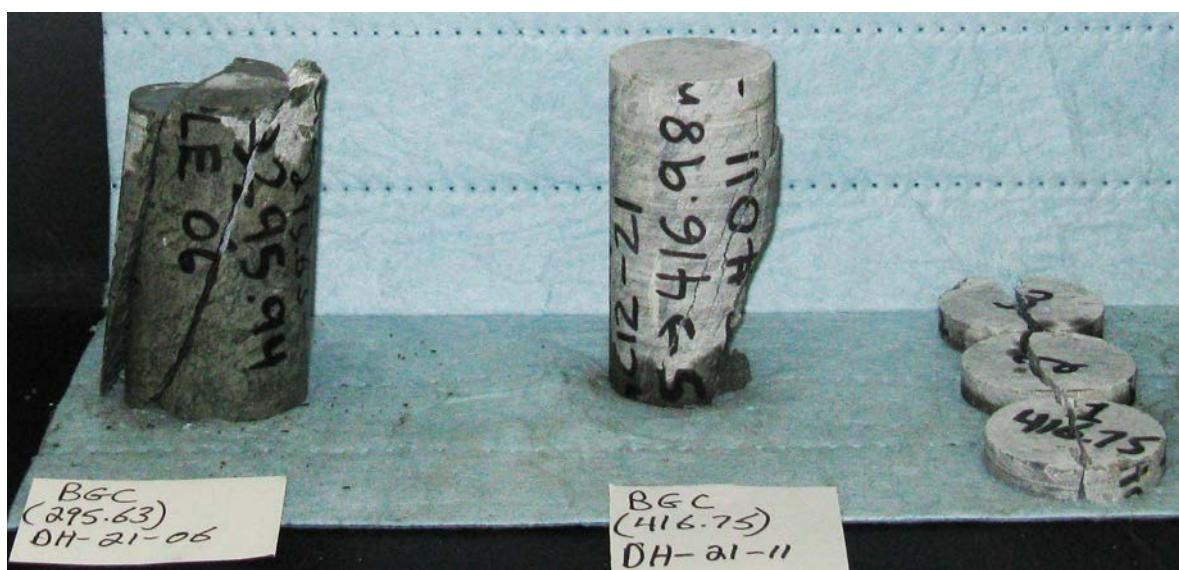
**Post-Test Direct Shear Sample Photographs**
