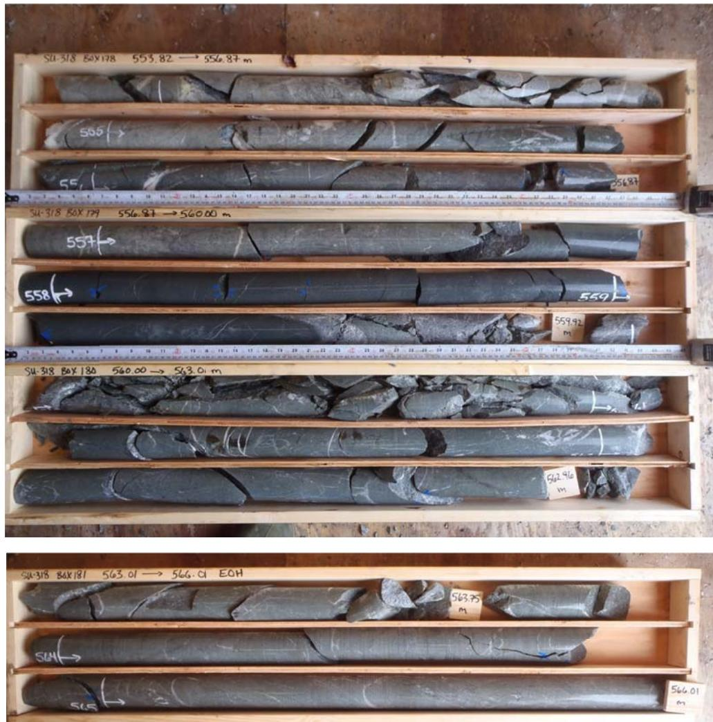
**Photograph G-2. Core Box Photos Showing Fault-disturbed Zone and Transition into Less Fractured Rock Below Fault Zone in DH-BGC12-23 (SU-318).**
