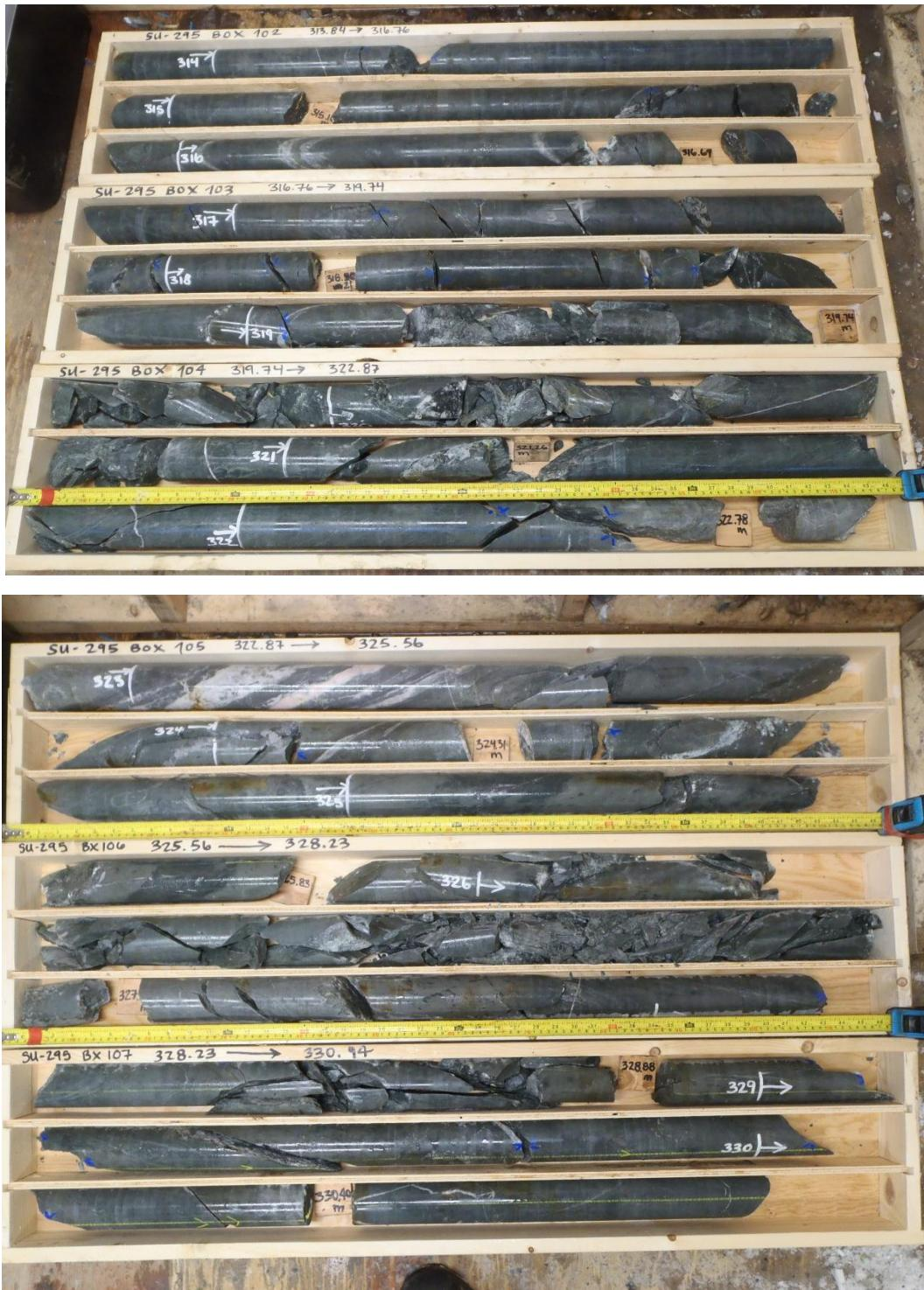
**Photograph 6-1. Core Box Photos from DH-BGC12-20 Showing Abrupt Transition into and out of Fault Disturbed Zone**
