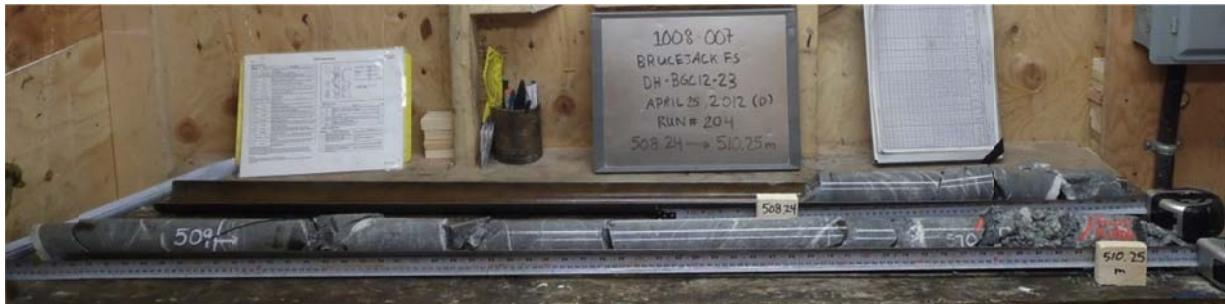
**Photograph G-5. 'Worst Case' Fault Discontinuity at 510.06 m in DH-BGC12-23 (100 mm Fault Gouge, Crushed Rock, and Broken Rock Infill) in Relatively Undisturbed Length of Core.**
