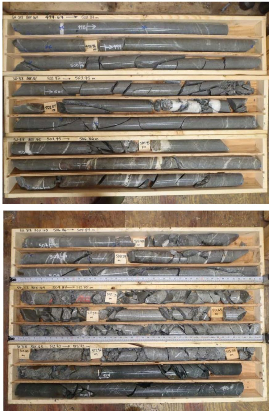
**Photograph G-1. Core Box Photos for DH-BGC12-23 Showing Transition from Decreasing RQD Values Beginning at 500 m Depth into Fault Zone at Approximately 507 m. Bottom Three Core Boxes are Illustrative of Typical Fault Zone Core.**
