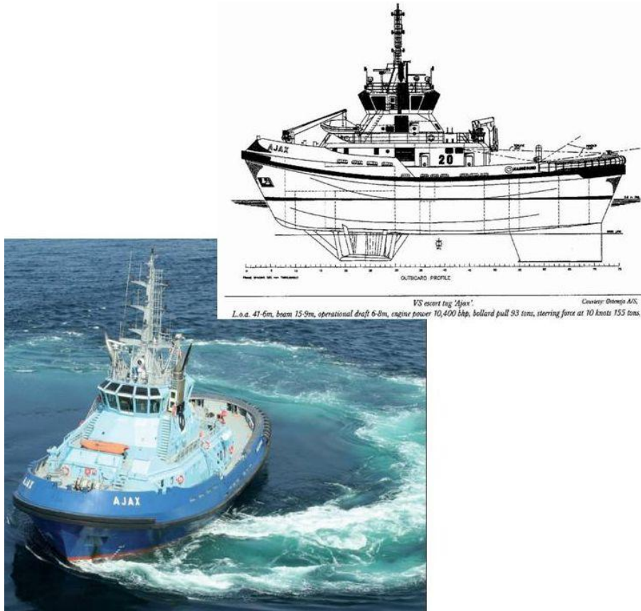
Figure 3-1: Typical views of an VS Tug (source: Østensjø and Voith Schneider)
