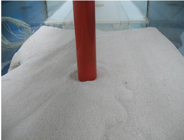
Figure 6-2: Single Pile Scour Test [28]
