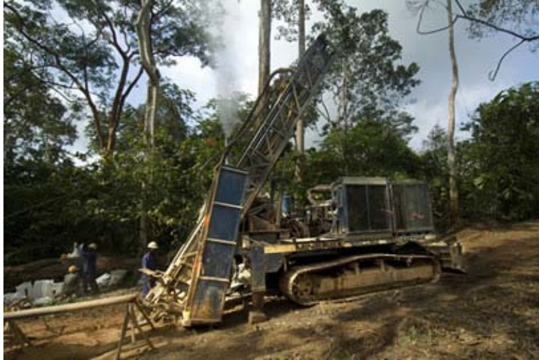
Figure 4-3: Typical Drilling Rig on Tracks (www.minerex.com)
