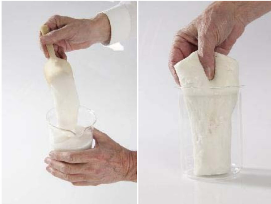
Figure 4-4: Water Gel Explosive Before and After Sensitizing ( www.maxam.net )
