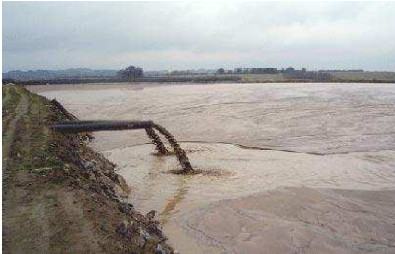
Photo 2-1 Deposition of Tailings Slurry at Glebe Mines, Derbyshire, England (© Jon Engels)
