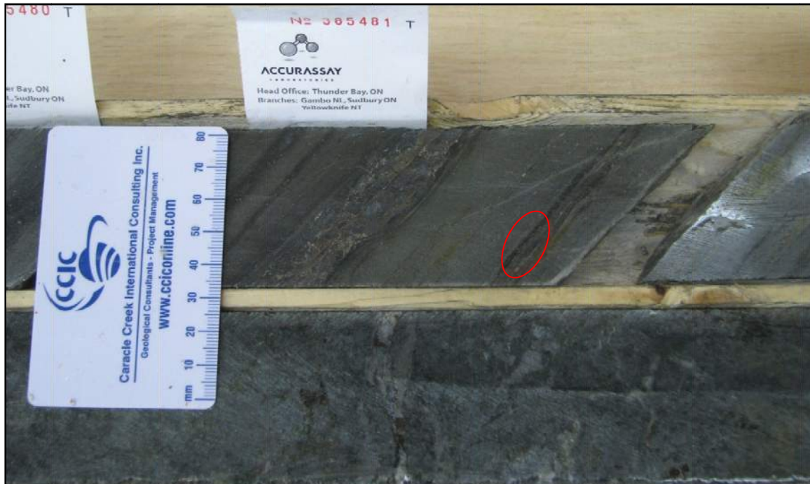
Figure 7-12. High-grade gold mineralization with flakes of visible gold (VG) in a strongly altered section in felsic metavolcanic (biotite-muscovite schist) from the Main Zone (TL08-15, 50.8 m).
