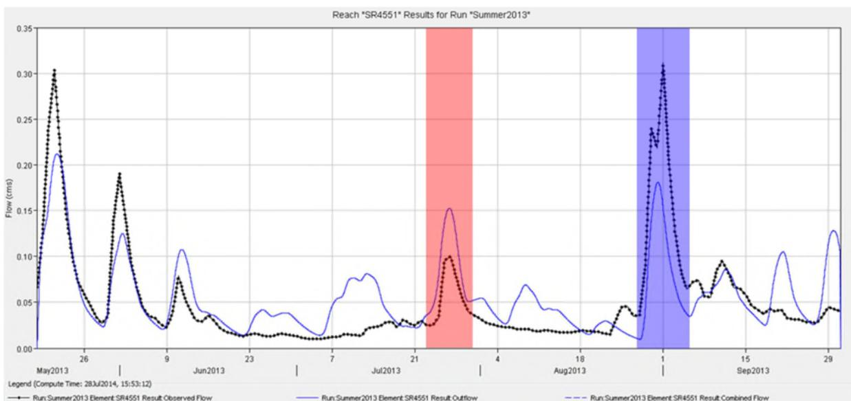
**Figure 3-3** 2013 Summer model calibration results for monitoring station TL1A (SR4551) at the Goliath Gold Project. Simulated flow is shown as solid blue lines while measured flows are shown as black dotted lines. The red highlight is the response to a July 25, 2013 rainfall event (28.1 mm) while the blue highlighted is a response to an August 29, 2013 rainfall event (43.0 mm).
