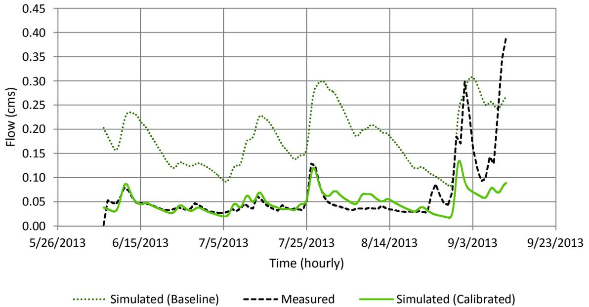
**Figure 3-4** Measured, baseline simulation, and calibrated simulation results for monitoring station HS4 (NR4658-2) at the Goliath Gold Project.
