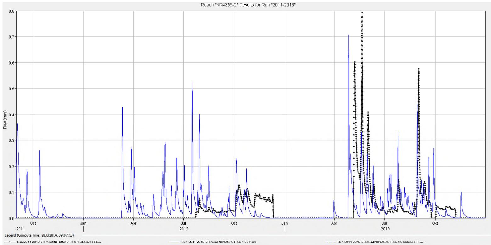
**Figure 3-2** Simulated results versus measured data for monitoring station HS7 (NR4359-2). Simulated flow are shown as solid blue lines while measured flows are shown as black dotted lines.
