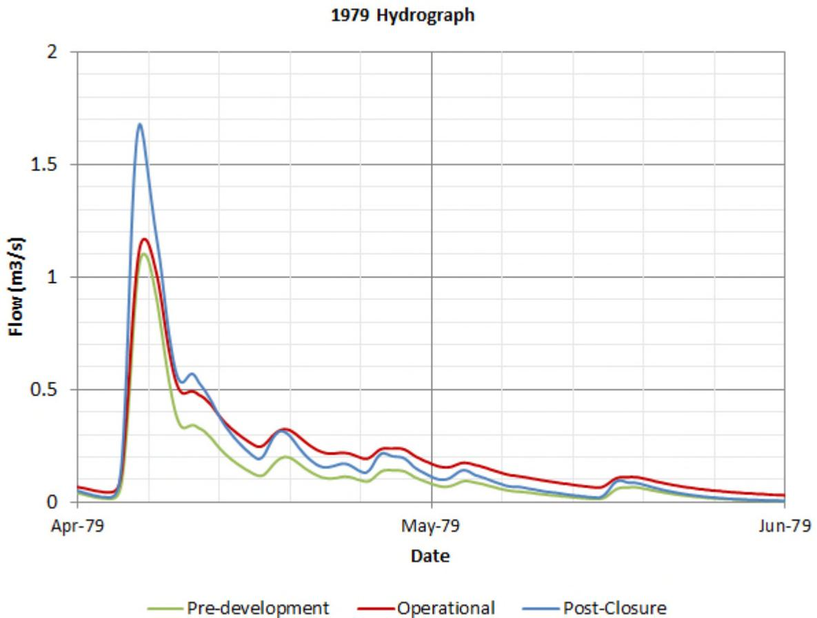
**Figure 4-3** 1979 spring freshet hydrograph for Blackwater Creek at the Goliath Gold Project.
