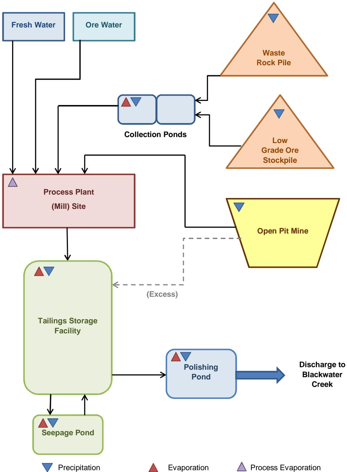
**Figure 3-6** Site Water Balance Flow Chart
