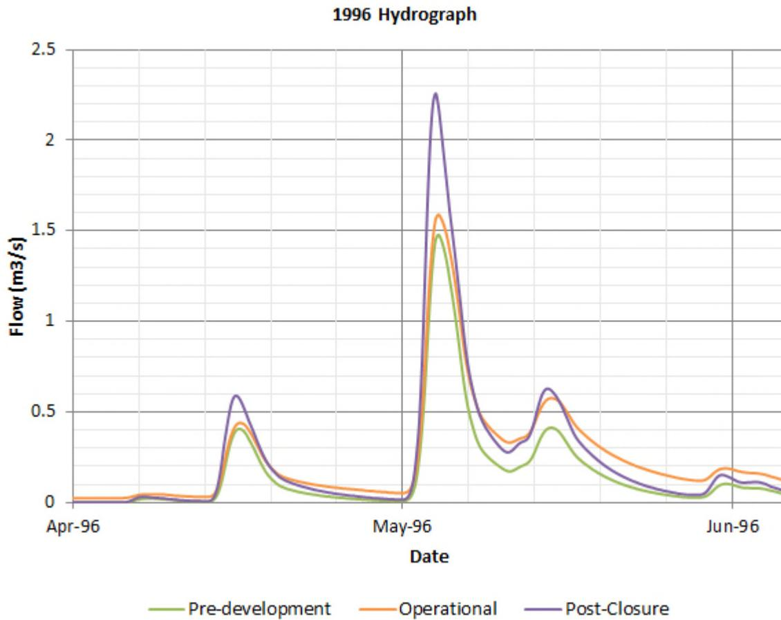
**Figure 4-5** 1996 spring freshet hydrograph for Blackwater Creek at the Goliath Gold Project.
