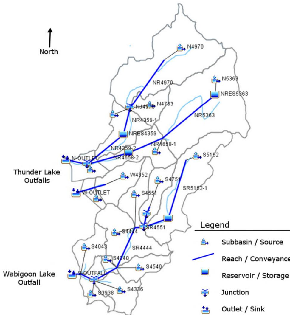
**Figure 3-1** Diagram of the subbasins and model components included in the HEC-HMS basin model for the Goliath Gold Project.
