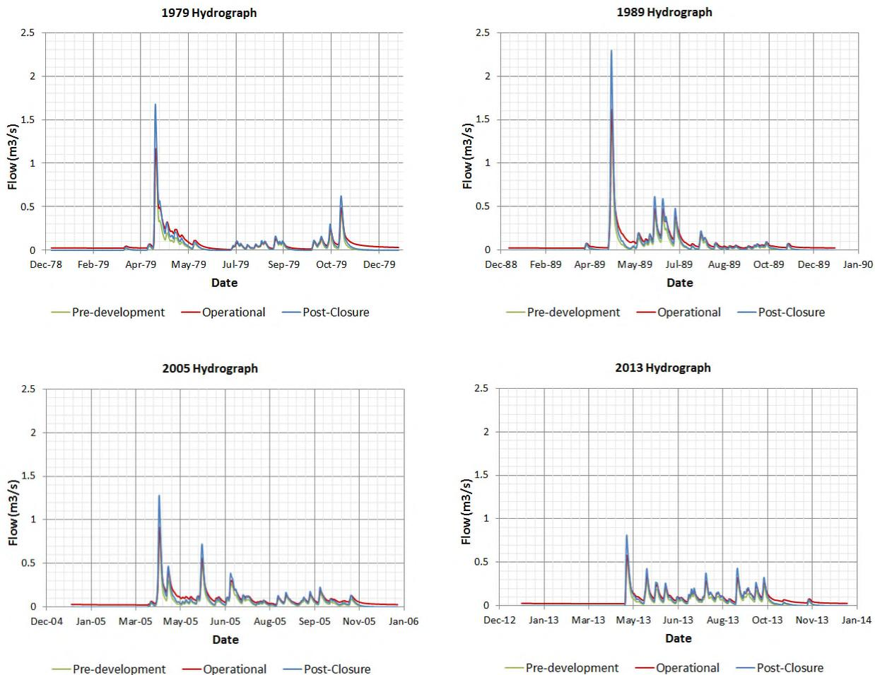
**Figure 4-2** Ten year low flow hydrographs extracted from the model for Blackwater Creek at the Goliath Gold Project.
