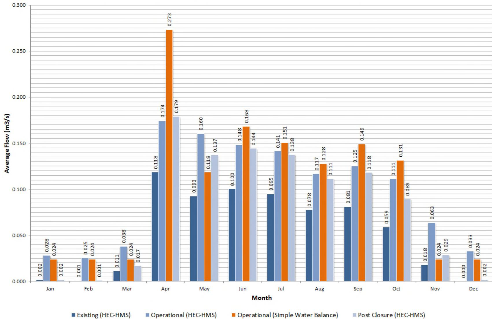
Figure 4-1 Monthly water balance for pre-development, operation, and post-closure phases of the Goliath Gold Project.
