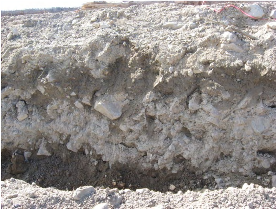
PHOTO 6 – Very Stiff Lodgement Till at the Site of the proposed Open Pit (WP 57)
