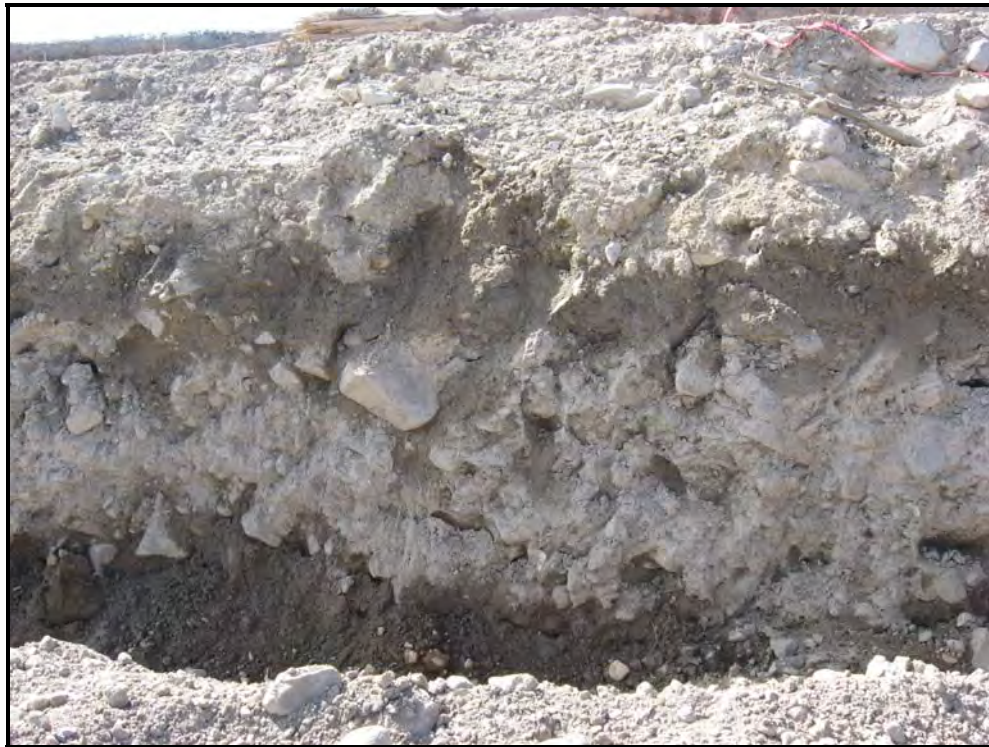
Figure 8.1 Exposure of Very Stiff Lodgement Till at the Site of the proposed Open Pit (WP 57)
