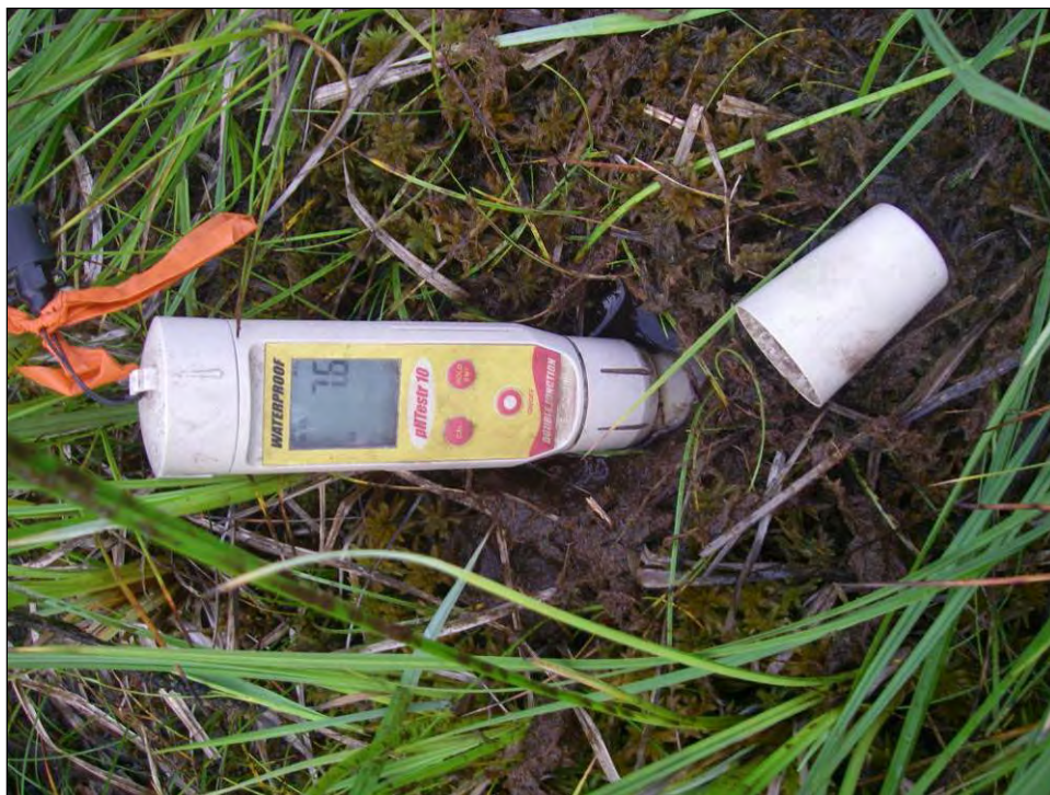
Plate 4.1-5. Oakton Instruments pH Testr 10 measuring pH of shallow groundwater in a soil test hole.
