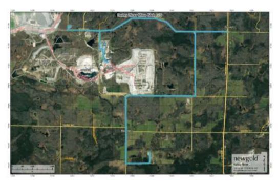
Figure 25 Road routes for Calcium Chloride application in 2021
