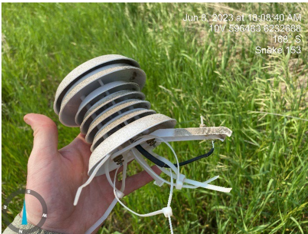
Photo B9: Destroyed temperature probe and solar shield at Snake Den 153 (Halfway River) on 8 June 2023.
