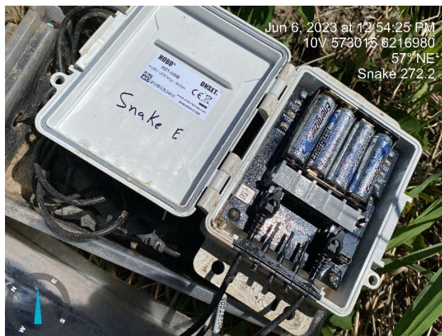
Photo B12: Water found within logger at Snake Den 272.2 (Peck's) on 6 June 2023.
