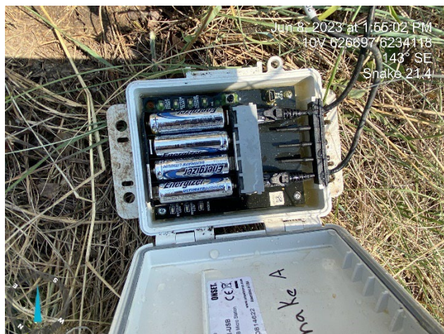
Photo B11: Water found within logger at Snake Den 21.4 (Dam View) on 8 June 2023.
