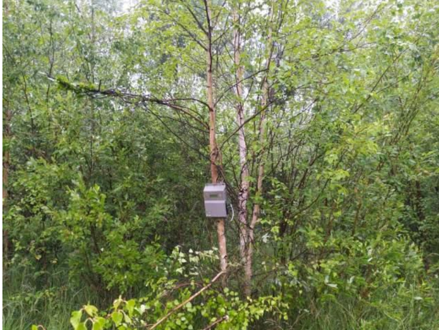
Photo 7 Example Deployment of an SM3 Autonomous Recording Unit with External Microphones within Wetland Habitats
