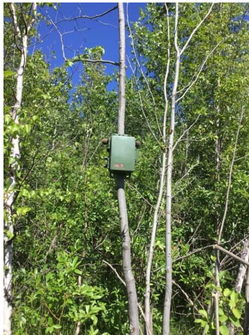
Photo 8 Example Deployment of an SM4 Autonomous Recording Unit with Internal Microphones within Wetland Habitats
