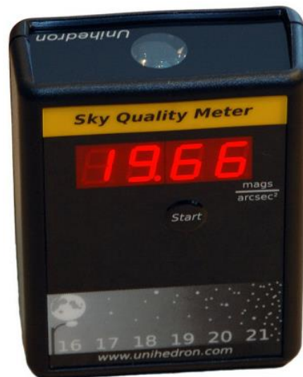
Figure 2.1.1: Sky Quality Meter by Unihedron
