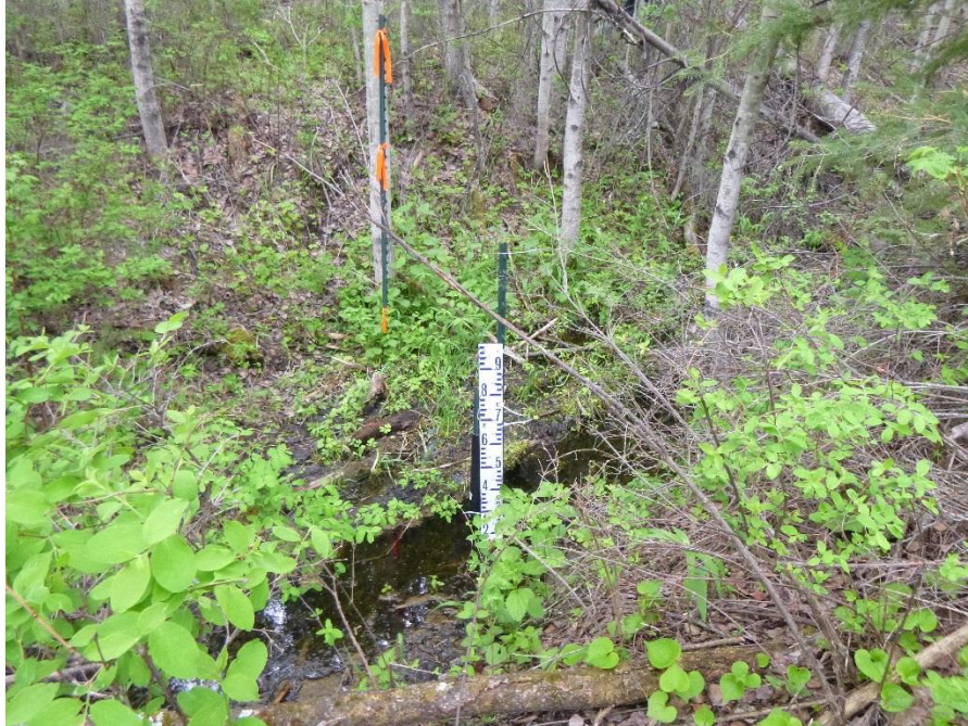
Photo 11. KEYNES hydrometric station and staff gauge on May 25, 2014. Note the poorly defined channel and abundance of large woody debris and organic matter.
