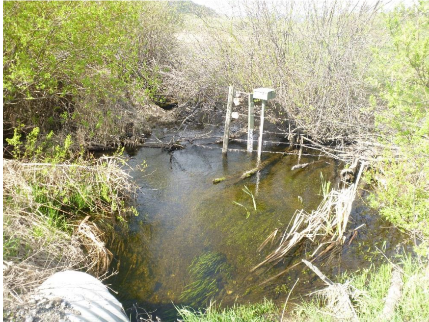
Photo 9. PETER hydrometric station and staff gauge on May 15, 2014.
