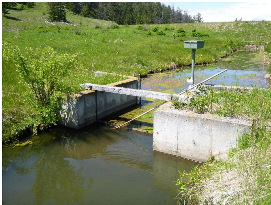
Photo 8. Looking upstream from JACSEEP hydrometric station towards the Jacko Lake low-flow outlet on June 1, 2014. Backflow conditions in the overflow channel have flooded the v-notch weir at the station, which prevents manual discharge measurement. Note that the red platform from which the outflow is controlled is visible in the background at the edge of the lake.
