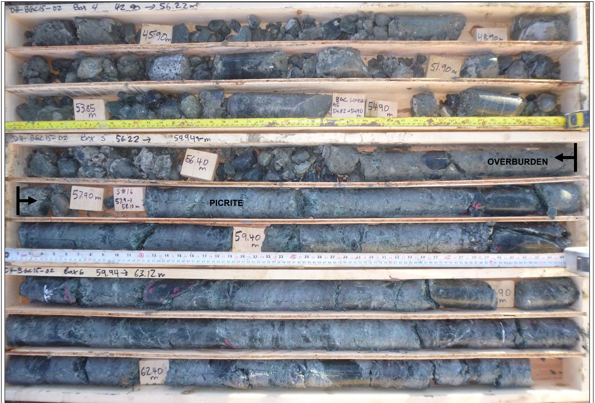
Figure 2 DH-BGC15-02: Very Poor quality, highly to completely weathered picrite
