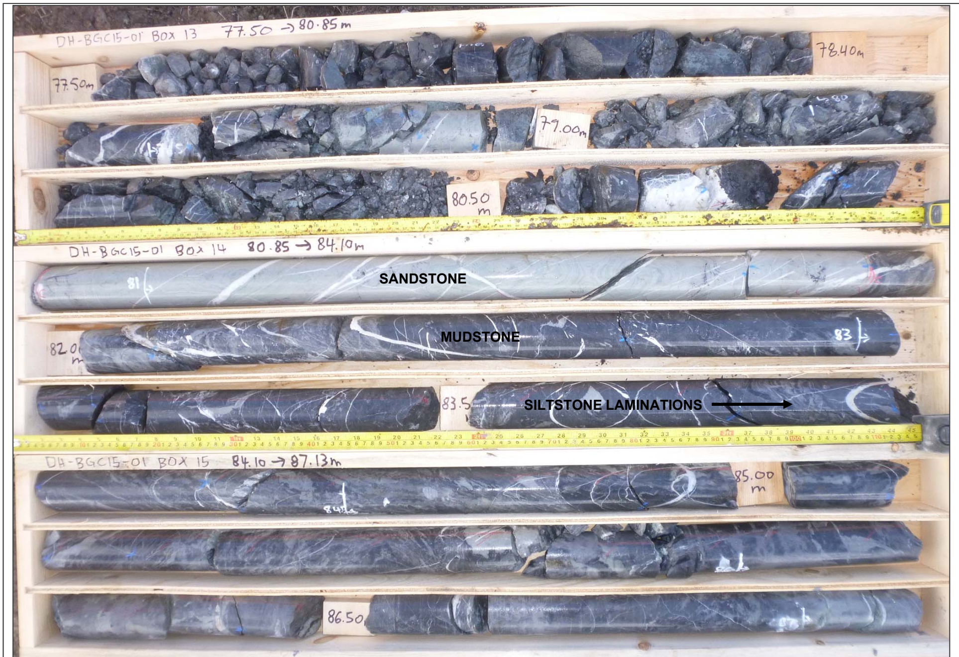
Figure 3 DH-BGC15-01: Poor to Good quality sedimentary rock including interbedded mudstone (dark grey) and siltstone (grey) with a layer of sandstone (light green).
