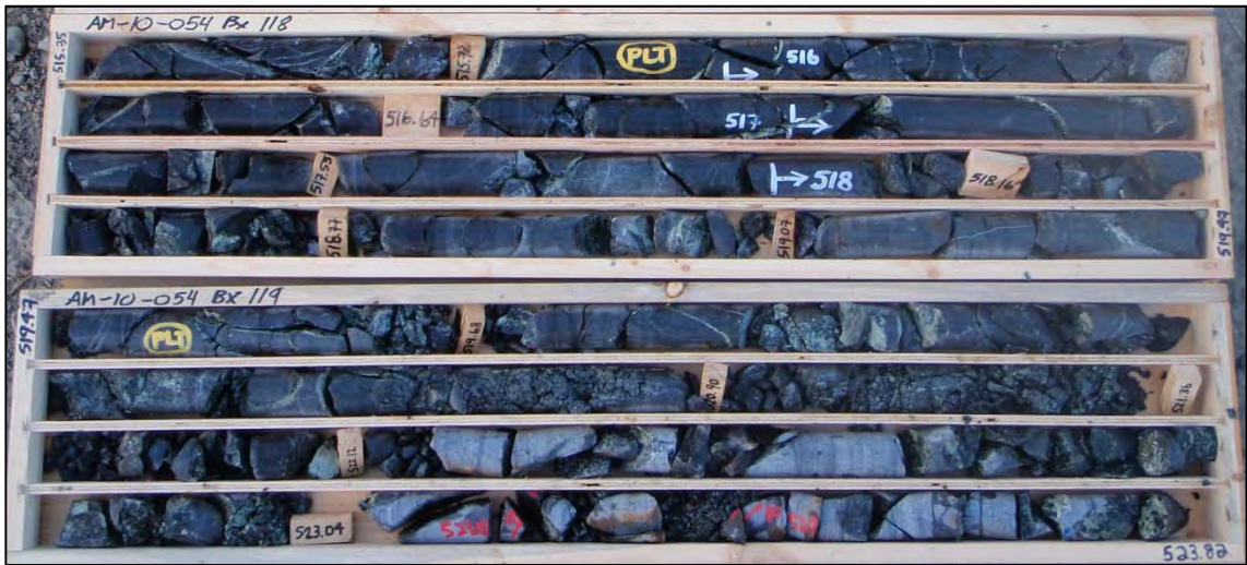
Figure F-5: AM-10-054 fault in PICR at ~520 m – zone of broken rock, fault gouge
