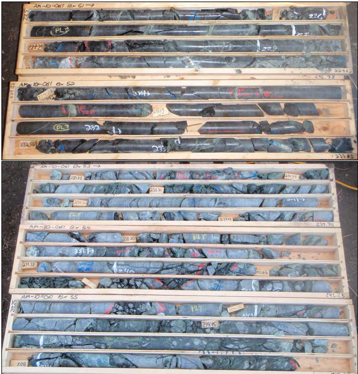
Figure F-8: AM-10-061 fault in PICR at ~233 m according to wireframe model. Core shows structures at 229.5 m and zone 241-245 m which could be the fault/ fault zone
