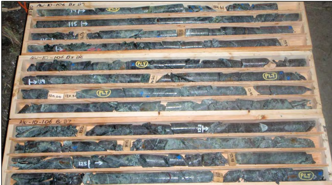
Figure F-9: AW-10-106 fault in IMH at ~119 m according to wireframe model. No obvious structure visible in core photos at 119 m, possible broken, weak, altered zone at 122-125. Rock is generally more broken, altered, and weaker than surrounding IMH.
