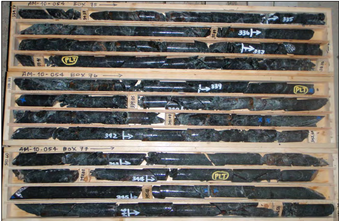
Figure F-4: AM-10-054 fault in SLD at ~339-343 m – zone of weak, broken rock
