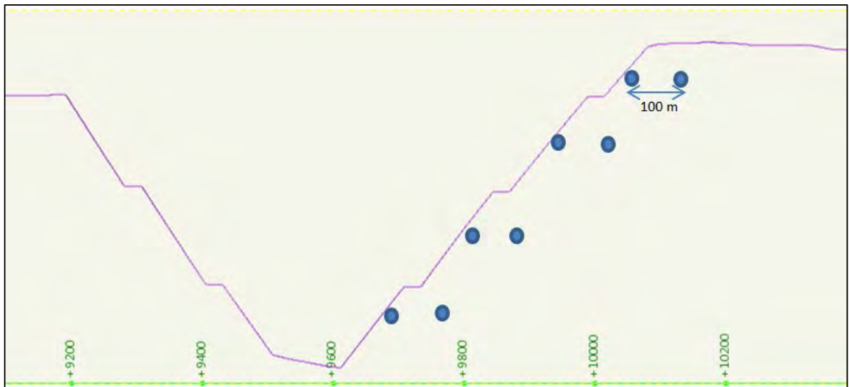
Figure 7-5: Cross section showing an example of history point locations within the pit wall
