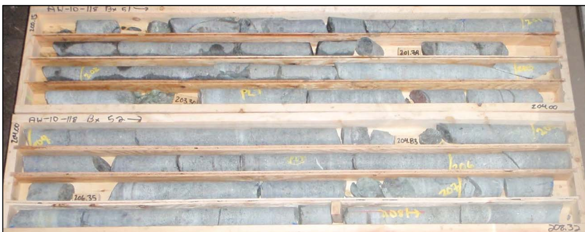
Figure F-10: AW-10-118 fault in IMH at ~205 m. Fault not obvious in photos- but structure with red iron staining (203.7 m) may indicate water bearing structure, which may be fault related
