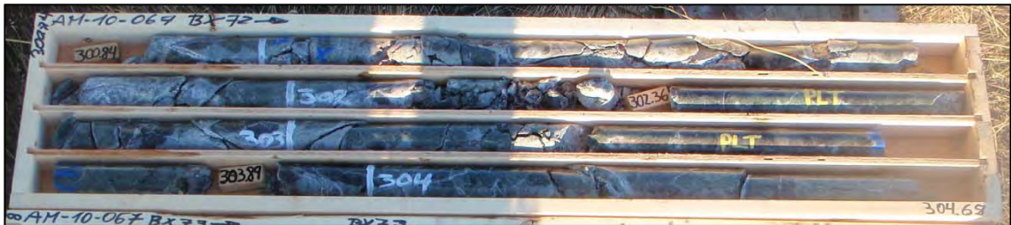
Figure F-6: AM-10-067 fault in SLD at ~300 m – fault gouge filled structure; rock appears more altered in immediate vicinity of fault
