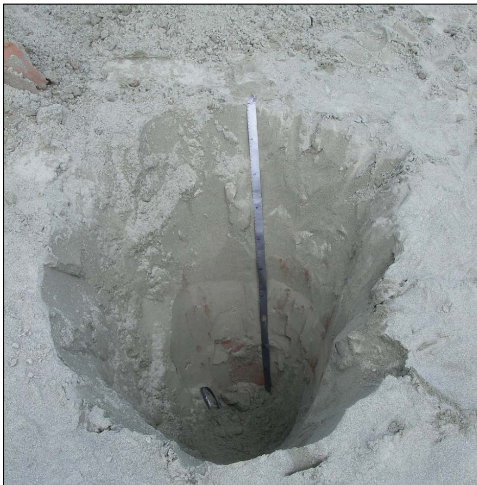
Figure 2-2: Photograph of a test pit constructed in the historic Ajax tailings
