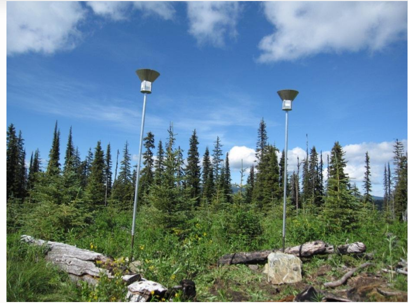
Dust Monitoring Station
