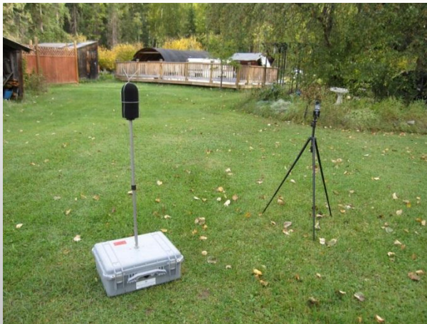
Portable Noise Monitoring Equipment
