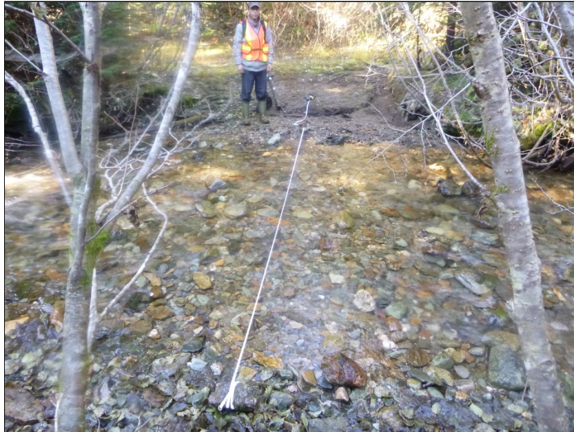
PHOTO F4 – Harper-Creek hydrology station (HARPER2), current meter measurement
