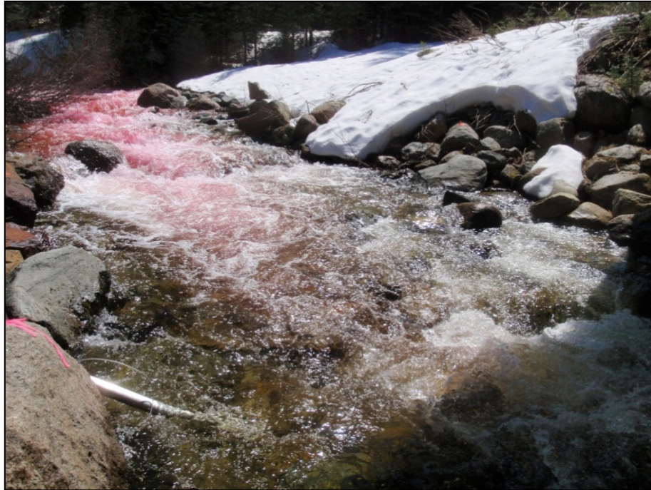
Figure 3.4 Dye Slug Injection Discharge Measurement at OP
