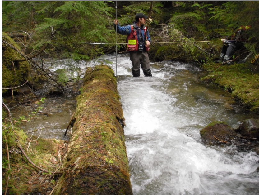
PHOTO B4 – Baker-Creek hydrology station (BAKERUS), current meter measurement
