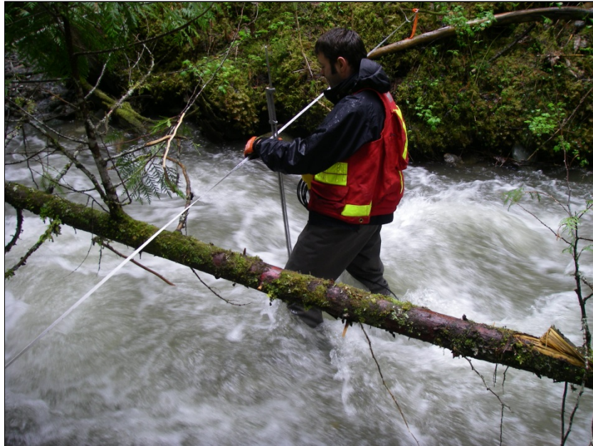
PHOTO C4 – Jones-Creek hydrology station (JONESUS), current meter measurement
