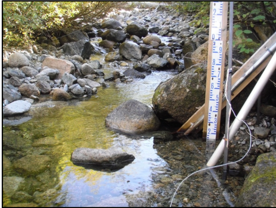
Figure 3.1 TSFDS Gauging Station looking upstream during low flow conditions ( <0.01 \text{ m}^3/\text{s} )
