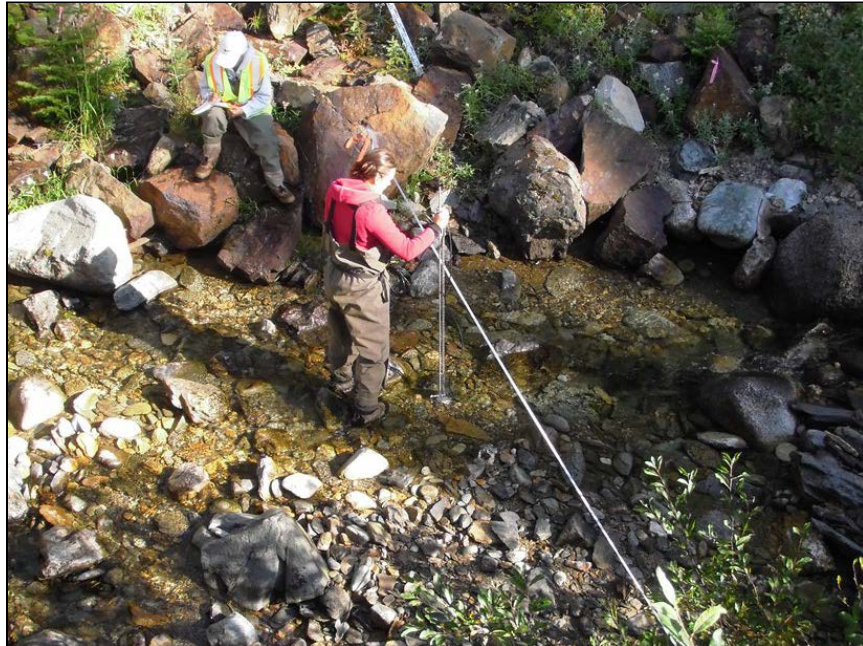
PHOTO D4 – P-Creek hydrology station (OP), current meter measurement
