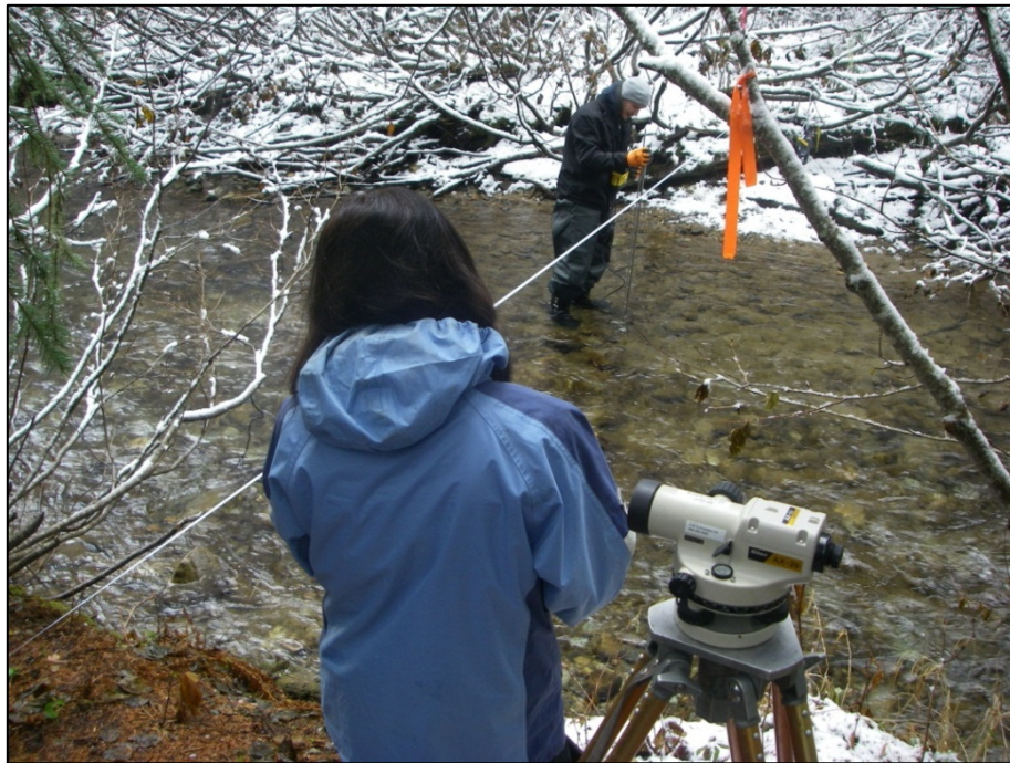
Figure 3.3 Velocity-Area Discharge Measurement at HARPERUS
