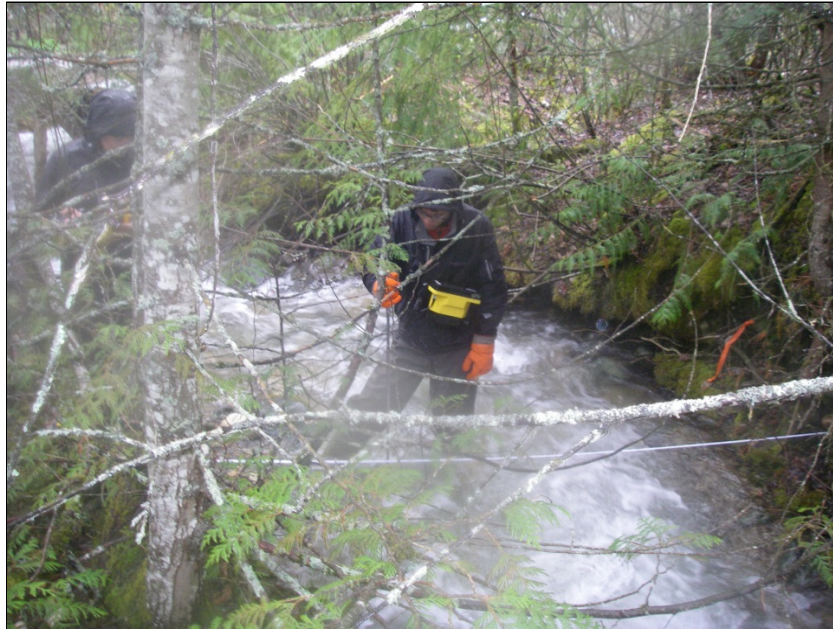
PHOTO A4 – Baker-Creek hydrology station (BAKER), current meter measurement
