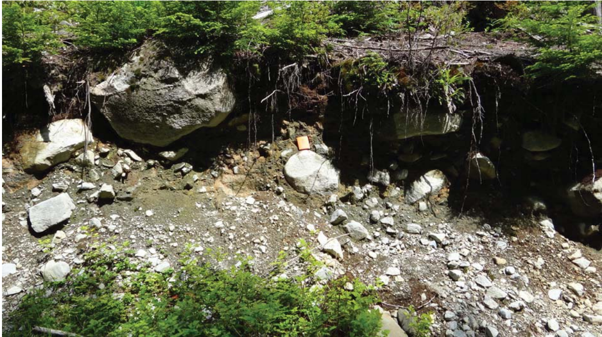
Photo 2: G063C3UW area, 2620 cutbank soils: variable thick till and colluvium.
