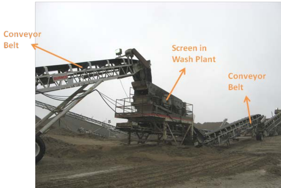
Photo 5: Screen 3 in the Wash Plant
