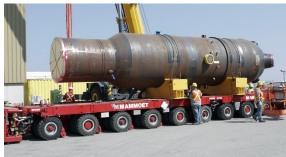
Figure 2-6: Steam Generator from Bruce A Station
