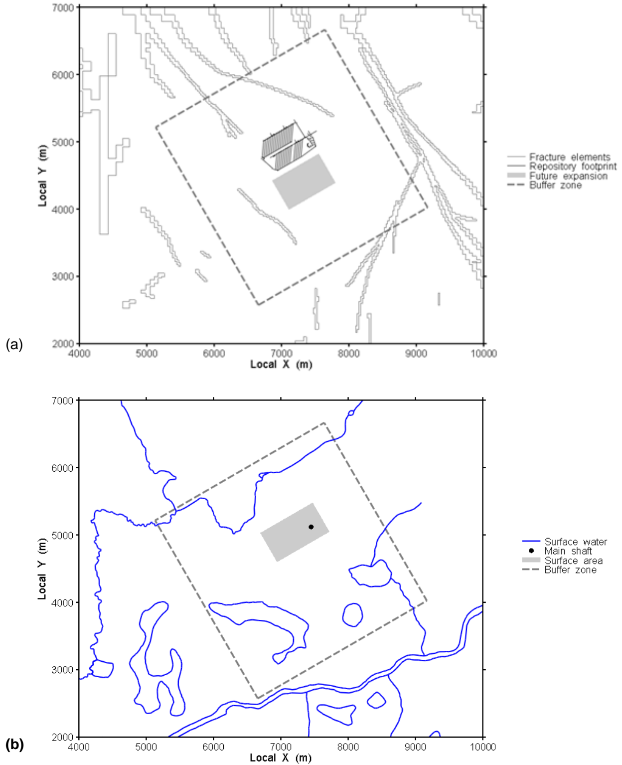
Figure 3-2: Illustrative DGR Placement in Crystalline Alternate Location. (a) Underground area, including expansion capacity, relative to main fractures; (b) Surface facilities area.
