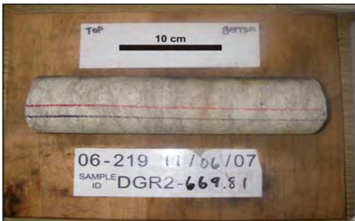
Figure 30: Core sample of argillaceous limestone from the repository horizon depth, Cobourg Formation, 669.8 meters below ground surface in borehole DGR-2. The limestone is dense with no visible pores, cavities, or fractures. (reproduced from DGR Geology TSD Figure 5.5.2-4)
