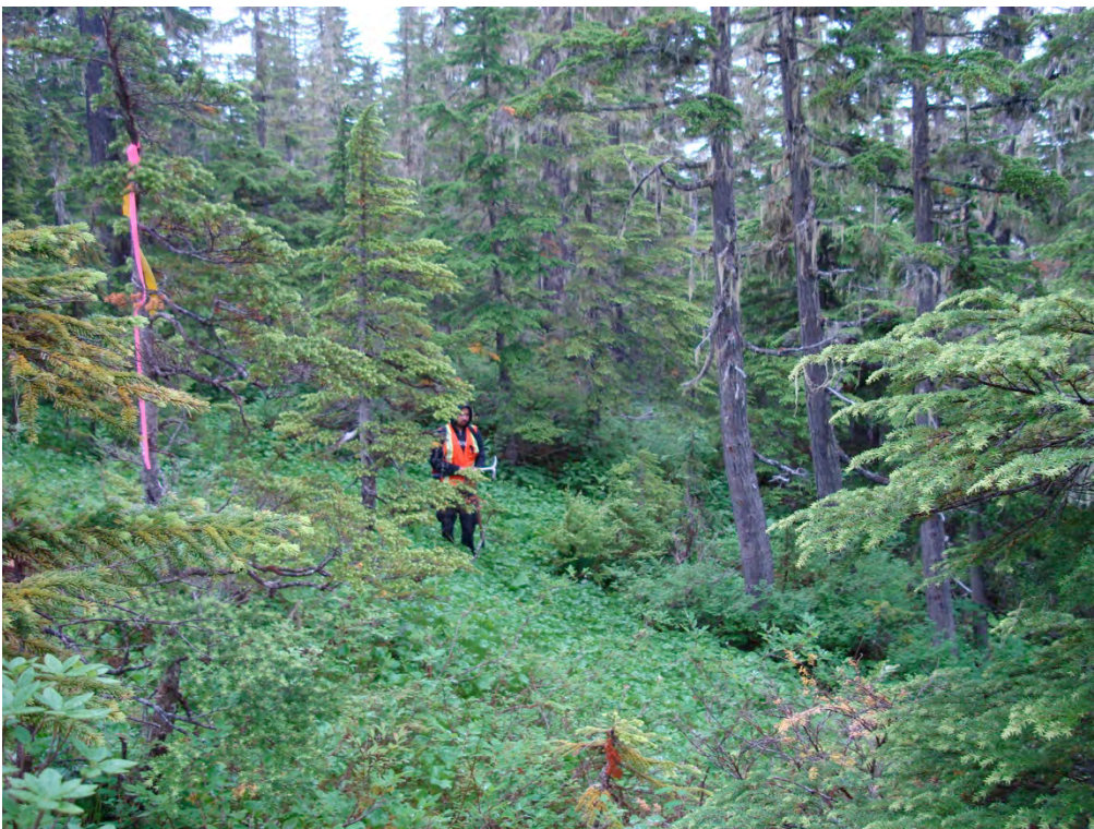
Figure 3 Organic soils on a forested slope. Leaning trees (photo centre right) show slope movement into a depression that breaks off steeply downslope.
