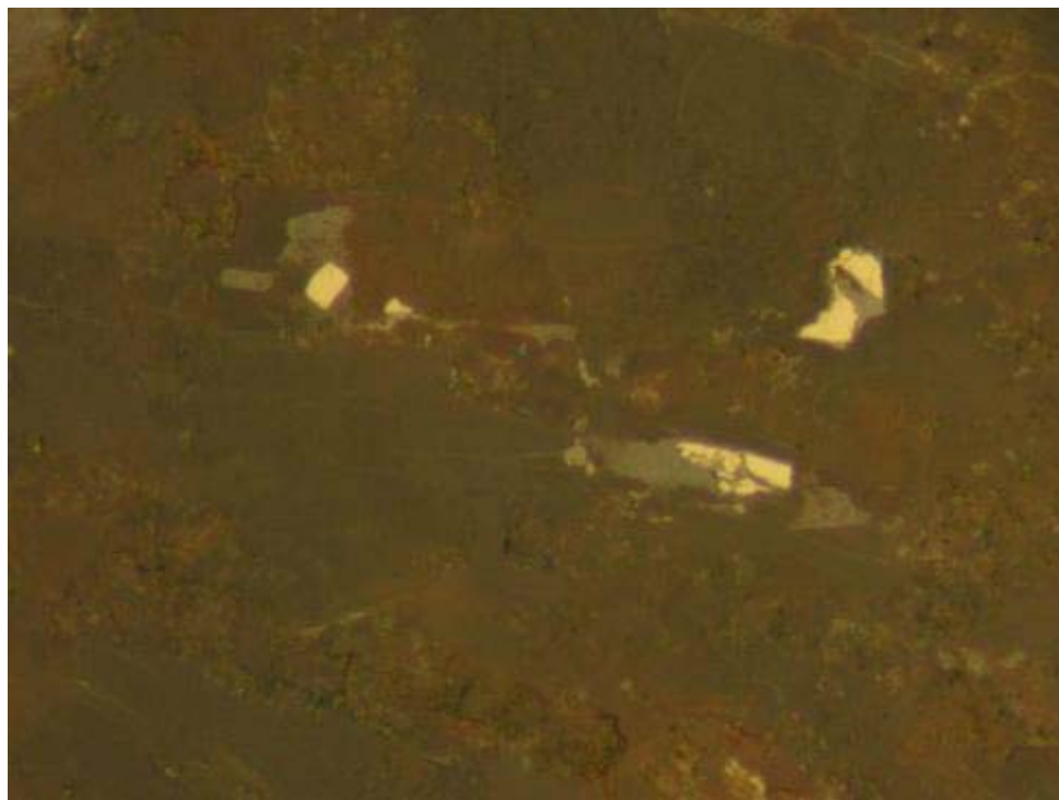
TP09-14-3: I) Disseminated pyrite partly replaced by Fe-ox material. RL. FOV \approx 0.2 mm.
