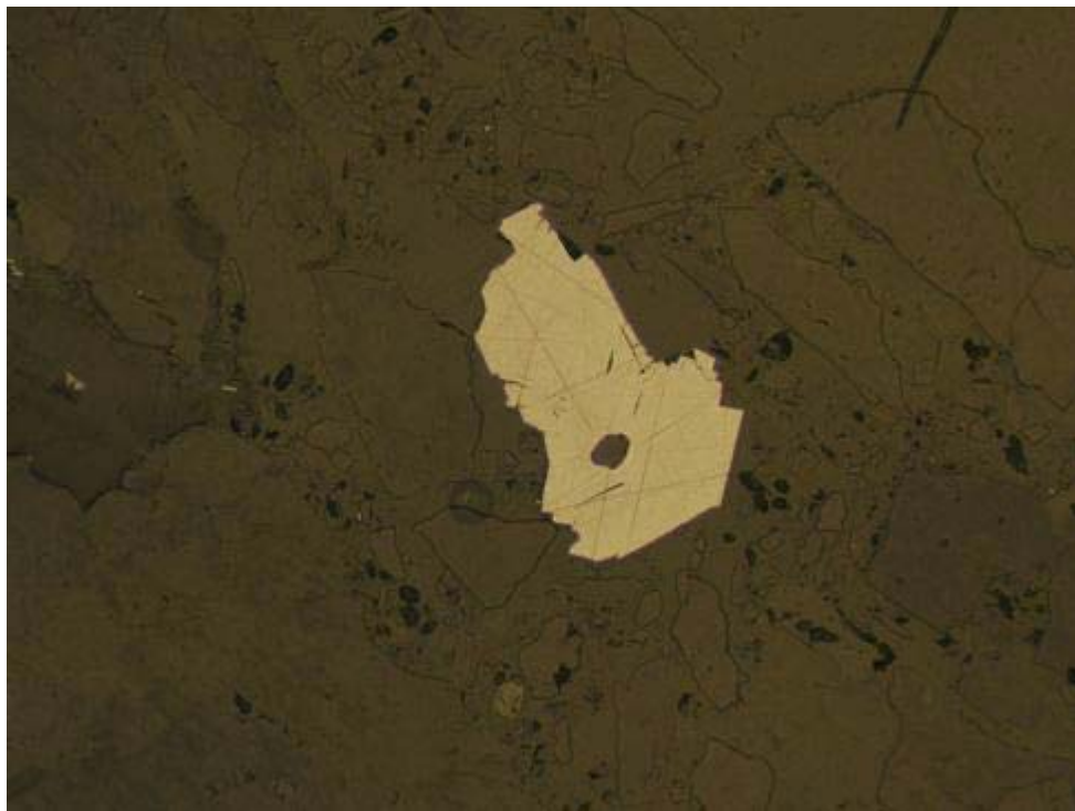
K08-22-144-147: G) Euhedral pyrite and platy molybdenite within granitoid chip. RL. FOV \approx 0.7 mm. H) Liberated galena aggregate. RL. FOV \approx 1.3 mm.
