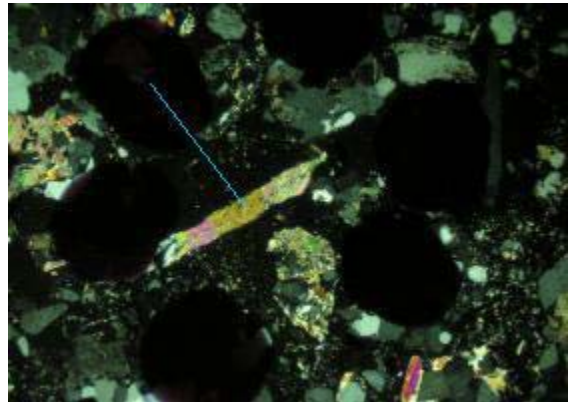
Circle #4 (XPL) FOV = 2.0 mm Blue line from ink dot to carbonate grain
