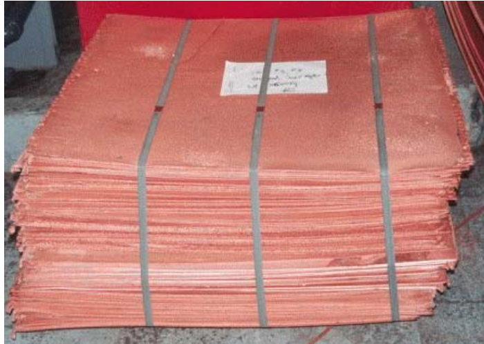
Figure 2 Copper cathode plate product
